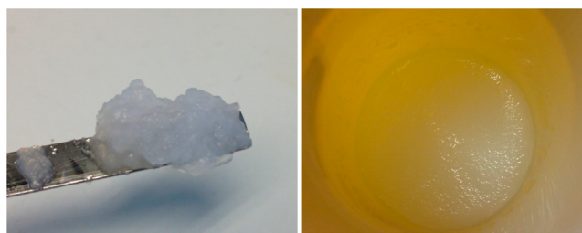
Figure 2. Solid product remaining after 1 h of microwave heating in pure methanol.
